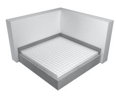
Install the perimeter strip and the Metro insulation
